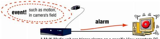
A Multi-Media unit can trigger alarms on a specific View operator's PC.
